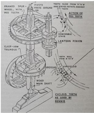
Examples of wooden gearing, and illustration of an improvement made by Rennie
